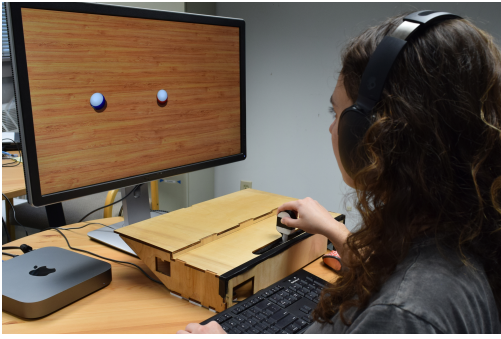
Fig. 2. A participant seated at the study setup with the haptic device in front of a computer screen. Users grasp the handle of the device, which provides vibrotactile feedback, while receiving audio cues via headphones.
